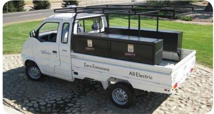
The Airport operates several low speed electric trucks and global electric motorcars (< 25 mph) which are ideal for short trips around the facility. (Photo: SCAS) (page 35 Oct 2011 CAP)
