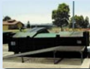
A ramp leading to the top of the dumpster makes it easier for disposal of the load.
