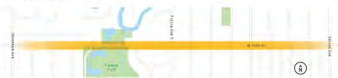
The West 58<sup>th</sup> Street portion of the project includes complete reconstruction of the roadway pavement, full installation of concrete curb and gutter, partial replacement of watermain and full replacement of water services, improvements to the sanitary sewer and storm sewer systems, traffic signal replacement at France Avenue, and construction of a 5-foot concrete sidewalk on the north side and an 6-foot concrete concrete sidewalk on the south side.
