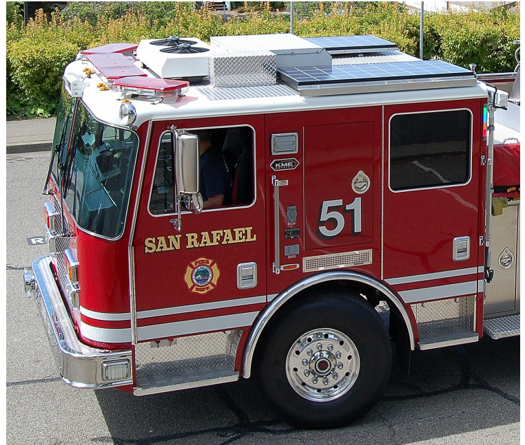
San Rafael Fire Department's Engine 51 is equipped with solar panels to charge the battery to run electronic devices on board.
