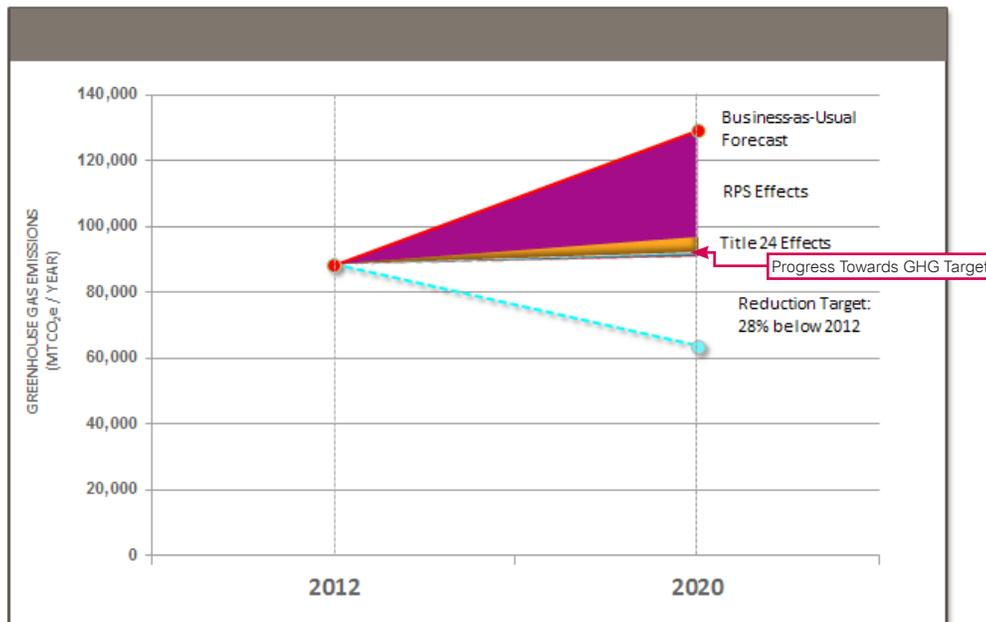
Figure B-5: Progress Towards Suggested GHG Reduction Target (Moderate EM Package and Moderate Demand Drivers)
