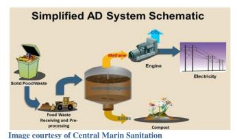
Anaerobic digestion is a natural process where bacteria breaks down organic materials such as food scraps, green waste, and other organic materials into "biogas" and fertilizer. It takes place in an oxygenfree environment in an enclosed container, or a natural environment sealed off from the air, such as a marsh, bog or wetland.
