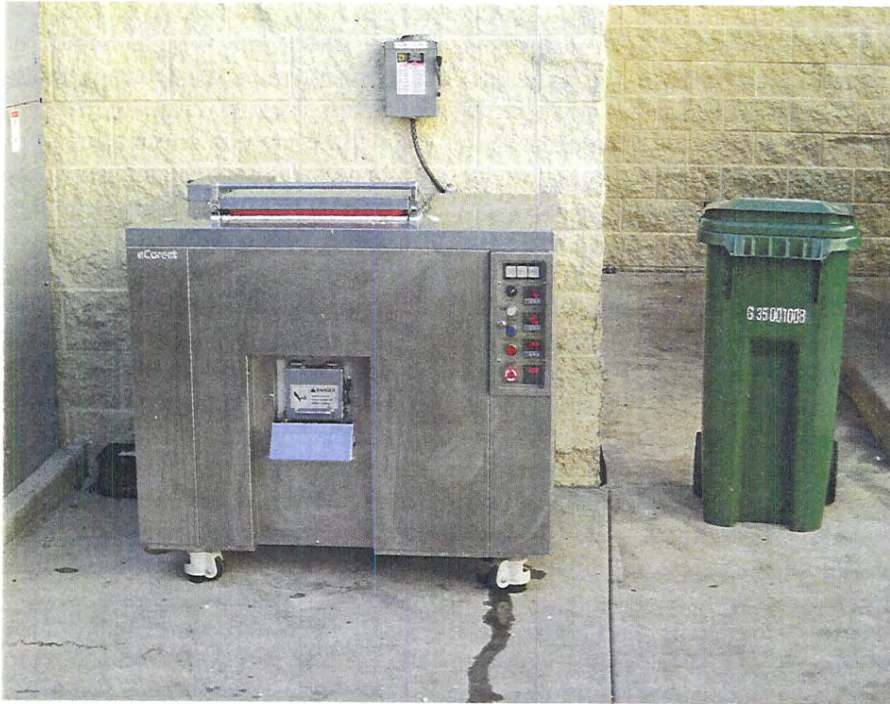
The eCorrect, an organics dehydrating machine that processes restaurant materials onsite
