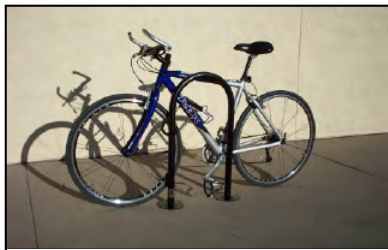
Example of Inverted U-Rack
