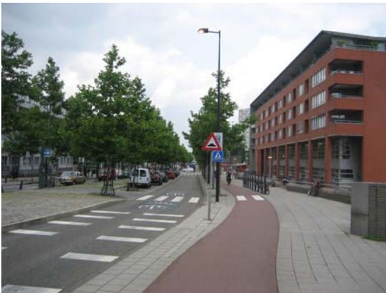
Photo 20: This bikeway in Amsterdam, Netherlands has separated bikes and pedestrians through colored brick and completely separates cars from bikes/peds.
