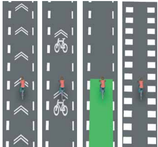
Crossing marking treatments from left to right: chevrons, shared lane markings, colored conflict areas, and elephant's feet
