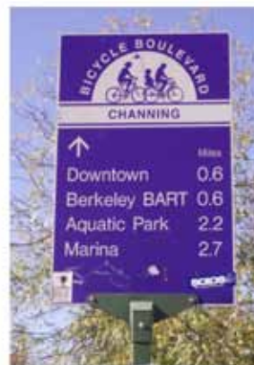
Wayfinding that includes distance and time can aid bicyclists in route finding.
