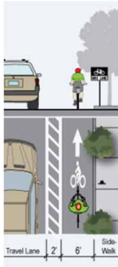
Buffers should be at least 2 ft wide because it is impractical to mark a zone narrower than that.
