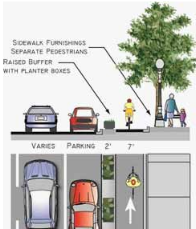
Recommended design with on-street parking, using a raised buffer with planter boxes for separation
