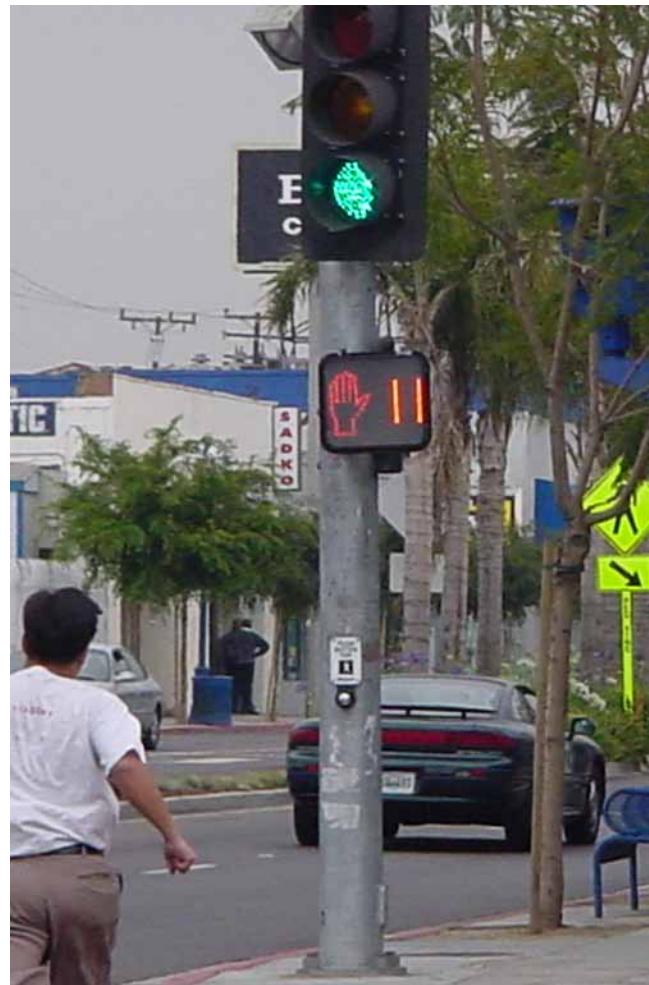
A pedestrian countdown signal displays the time remaining for pedestrians to cross
