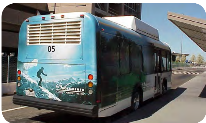
At Sacramento International Airport, the County replaced its fleet of almost 40 diesel buses with buses powered by compressed natural gas (CNG). (Photo: SCAS)
