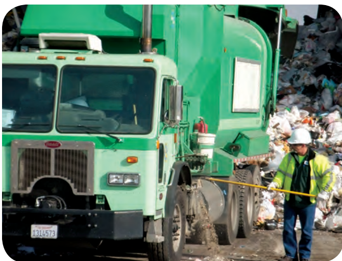
An automated collection vehicle ejects its load of commingled residential recyclables at the North Area Recovery Station. (Photo: DWMR)
