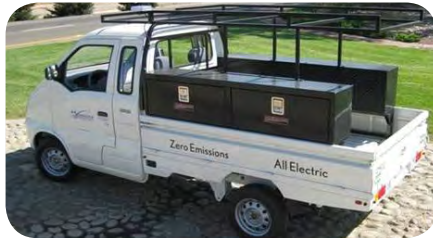
The Airport operates several low speed electric trucks and global electric motorcars (< 25 mph) which are ideal for short trips around the facility. (Photo: SCAS)
