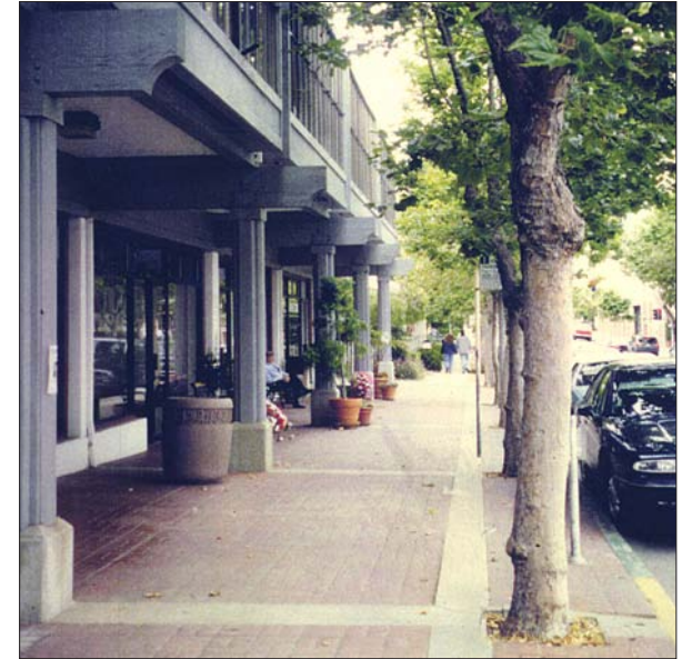
Where building overhangs occur, columns and streetscape elements placed below the overhang must not obstruct the walkway.
